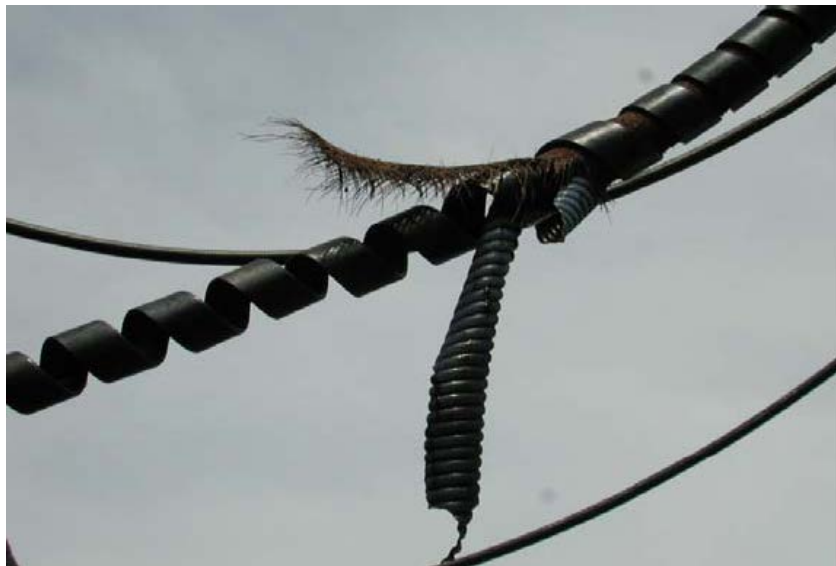
Ruptured chlorine transfer hose with its Teflon inner layer exposed; when the hose burst it ejected pieces of Teflon as well as other components of the hose.
