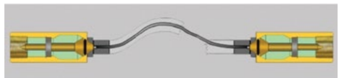
Hose Failure - Tear
