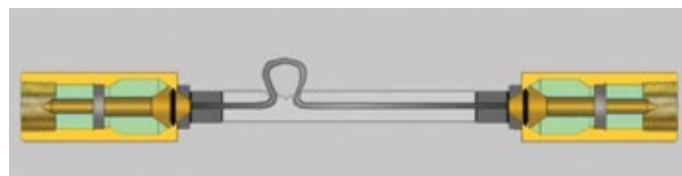
Valve Closed - Flow Shut-Off
