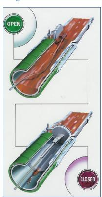
separates under a controlled condition and prevents product loss in the event of an emergency separation. The LifeGuard™ Tri-Bolt Breakaway Hose is designed to separate at any angle when subjected to a designated pull force. In case of separation, its patent pending design assures that not less than two bolts will separate causing the internal valves to engage and the piping to remain intact with flow stopped on both ends of the hose.
